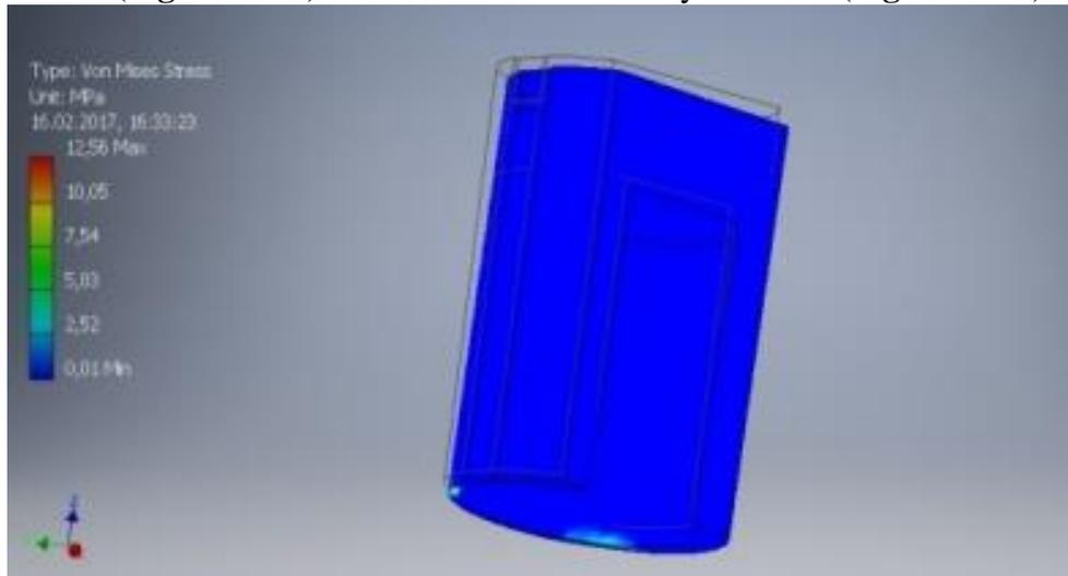
**Figure no. 7. Maximum von Mises stress on PM1 in case of implant supported RPD with attachments without M2**
