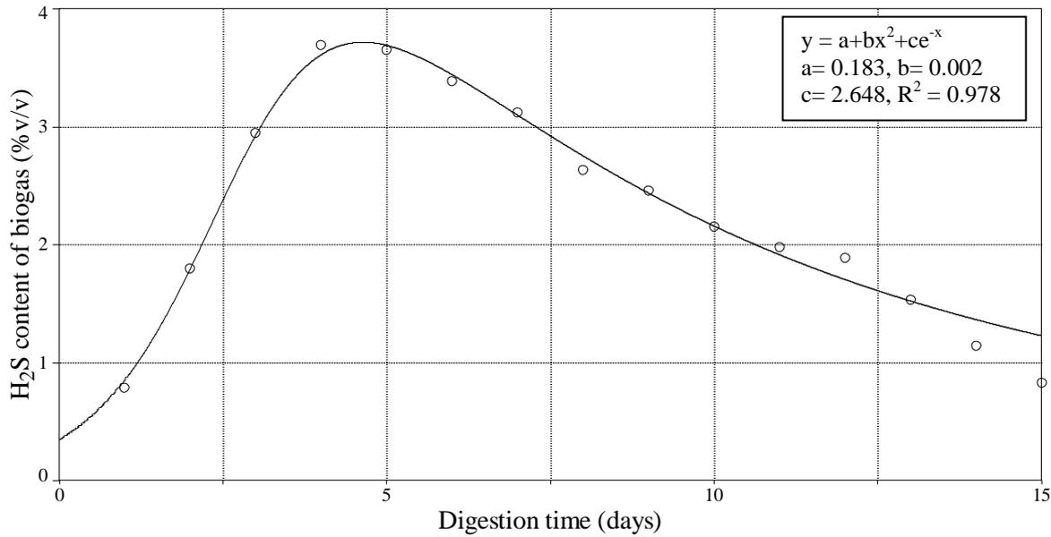
Figure 4. Daily H<sub>2</sub>S content (% v/v) of the produced biogas
