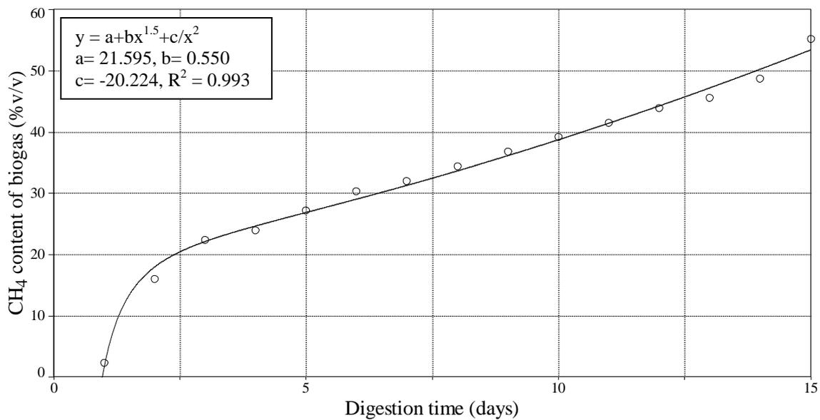
Figure 3. Daily CH<sub>4</sub> content (% v/v) of the produced biogas
