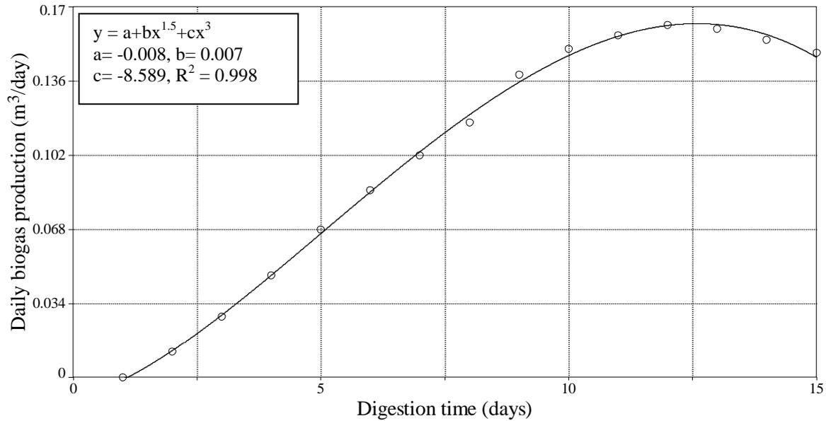
Figure 2. Daily biogas production during the anaerobic digestion process
