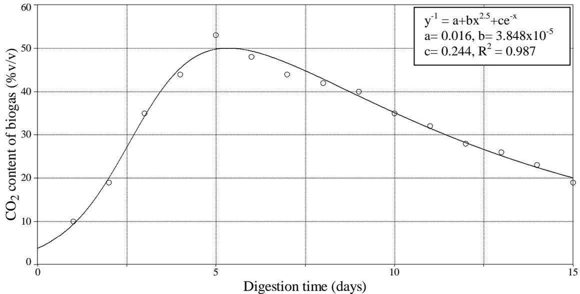
Figure 5. Daily CO<sub>2</sub> content (% v/v) of the produced biogas
