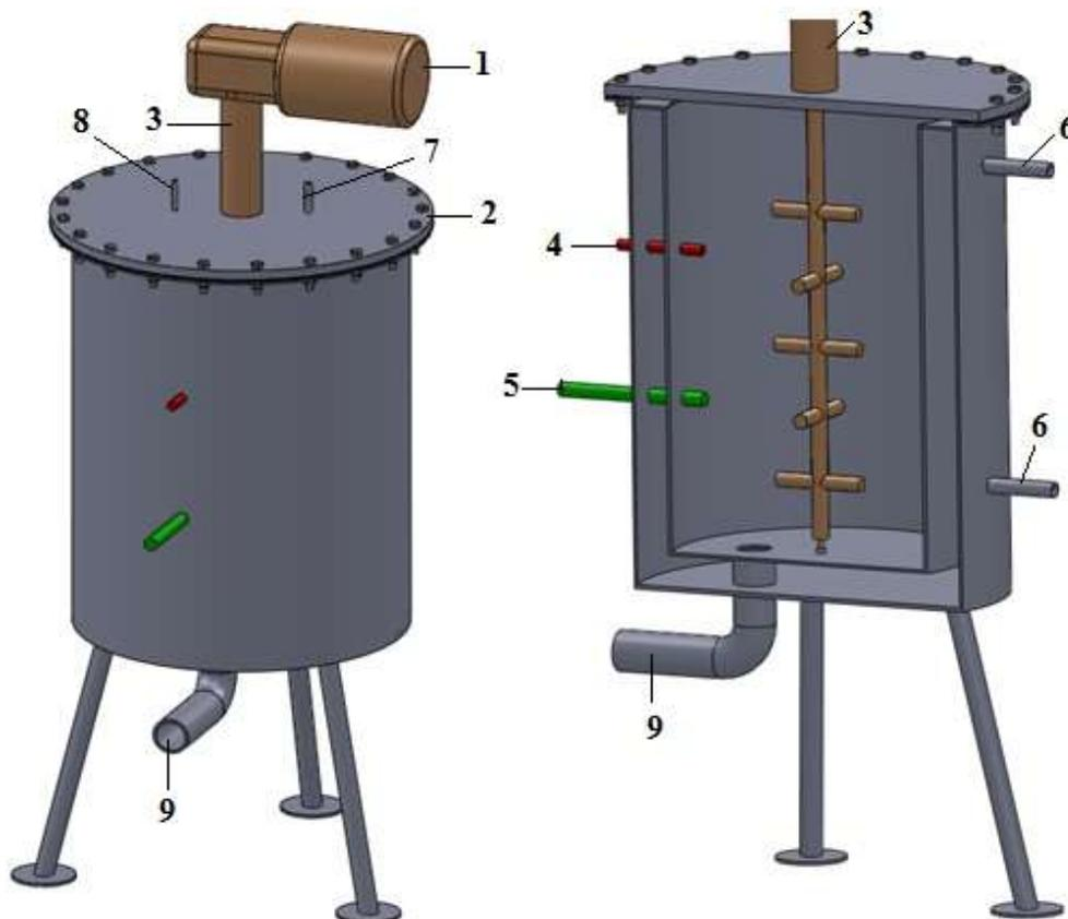
Figure 1. Design of anaerobic digester used in the experiment
