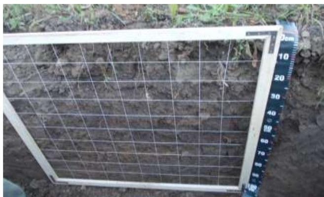
**Figure 1.**Metrical frame for tree-root measurements
