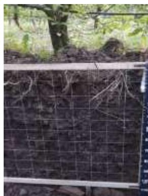
**Figure 3.** Metrical frame for tree-roots measurements in Florina cv/M9
