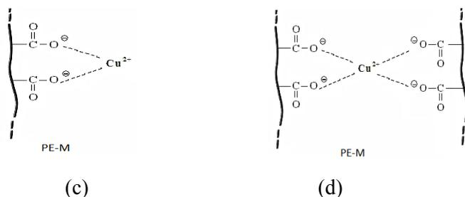
**Figure 3.** Structure of poly(MVE-MA) (a); PAA (b); PE-M (c) and PE-M-PE (d).
